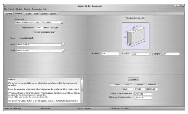
On the right side, enter the overall dimensions of the structure (Location) and click Update to get the expected incidence values for the Structure.
