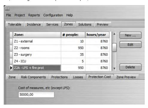
Note: in the Hospital example, the standard brings the cost of fire protection to zone 3 (Rooms), as in the figure above, but they bring a single cost for the shields in zones 4 and 5; in this example, we divide the value by 2 and put \$55,000 in each zone (see Total summation below).
