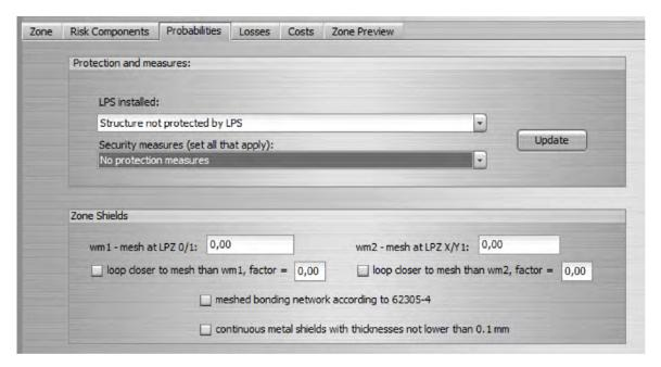
On the bottom panel, enter the shields between zones 0/1 and 1/2, if any.
