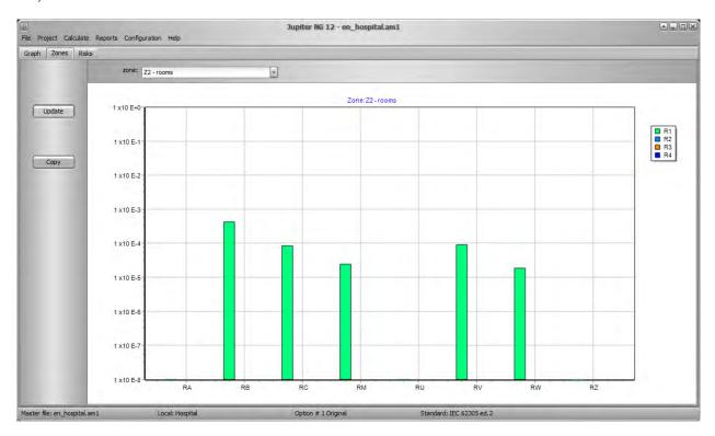
The Risk Report visually shows the proportions of Risks between the Zone, selecting a Zone, shows the distribution between the components of Risks for that Zone; this way, it is clear to the user which zones are more dangerous and which are the main components, that is, Jupiter shows graphically where it will be more efficient to adopt protective measures!
