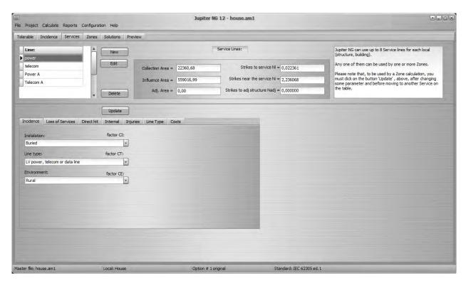
To enter each Service line, click New, provide the data and, in the tabs below, select the characteristics of the line; click Update to have the event numbers for the Service line, next to the Service and the adjacent structure (if any) calculated and stored in the file.
